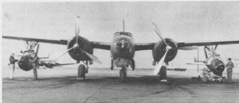
B-26 MOTHER SHIP carries two Ryan Firebees, one under each wing, in Holloman tests. Pilotless target drones are released by means of electric bomb salvo switch.
