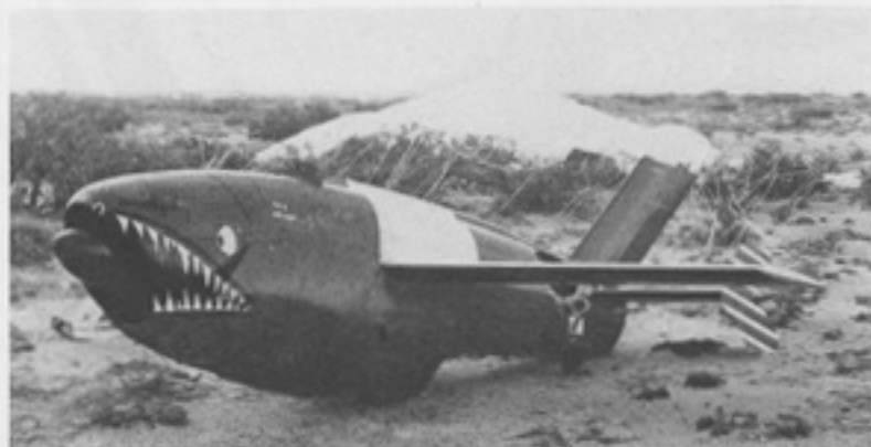
SAFE ON GROUND after parachute drop, Firebee waits for Air Force crane and trailer to pick it up, after which B-26 mother ship will launch second drone.
